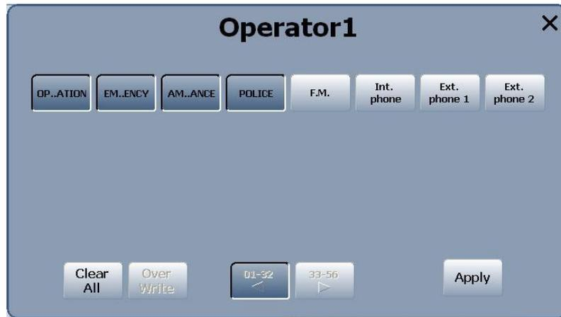
The selection/deselection of a channel is made by touching the toggle channel button. Here above, the "Operation", "Emergency", "Ambulance" and "Police" channels are selected as they appear in dark grey colour, one touch on one of these channel buttons will deselect the concerned channel which will then appear again in white colour. Touching the "Clear All" button will deselect all the channels.
