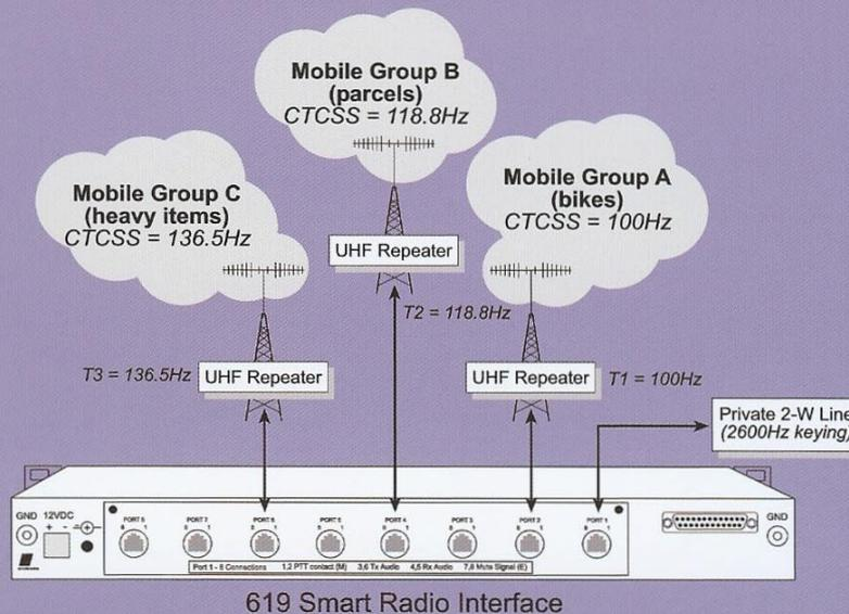
In this application the dispatch operator can command the 619SRI to cross link mobiles from different groups by controlling the CTCSS conversion facility in the bridge.
