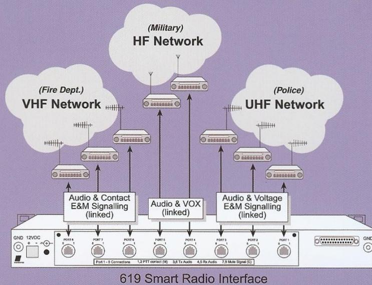
The 619SRI can act as a hub for radio networks utilising DHC, (Dynamic Hub Configuration), which allows the operator to dynamically change the system by sending a remote command sequence.
